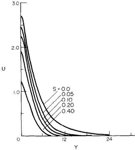
FIG. 2. Velocity profiles for an axisymmetric plume at  $Pr = 7.0$  and  $X = 100$ , for various values of the stratification parameter  $S$ .
