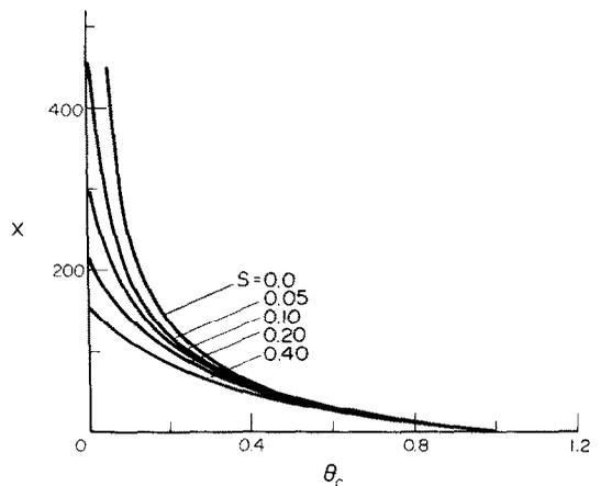
FIG. 5. Downstream centerline temperature variation in the plume at various values of  $S$  for  $Pr = 7.0$ .
