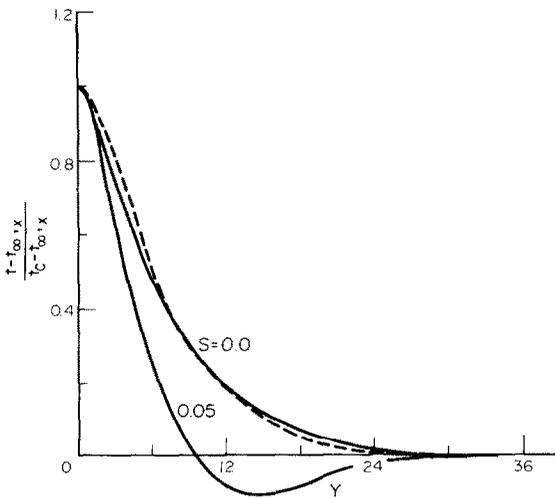
FIG. 3. Computed temperature profiles for the plume flow at  $Pr = 0.7$  and  $X = 100$ . --- temperature profile at  $S = 0$  from [10].
