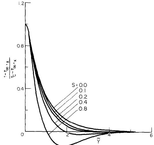
FIG. 7. Temperature distributions in an axisymmetric jet at  $Pr = 0.7$ ,  $X = 0.2$  and  $Gr/Re^2 = 0.47$  for various stratification levels.
