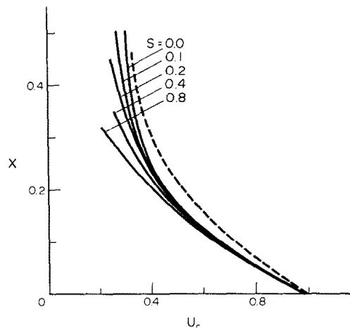
FIG. 11. Downstream variation of the centerline velocity in the buoyant jet at  $Pr = 0.7$  and  $Gr/Re^2 = 0.47$ . --- variation at  $S = 0$  for  $Gr/Re^2 = 0.94$ .
