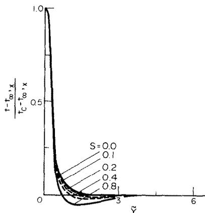
FIG. 9. Temperature profiles in the jet flow at  $Pr = 7.0$ ,  $X = 0.1$  and  $Gr/Re^2 = 0.47$ .
