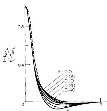
FIG. 1. Temperature profiles for an axisymmetric plume at  $Pr = 7.0$  and  $X = 100$ , for various values of the stratification parameter  $S$ . --- temperature profile at  $S = 0$  from [10]; - · - temperature profile for ambient temperature variation as  $X^{0.2}$ , with  $S_0 = 0.4$ .
