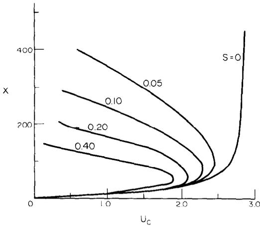
FIG. 6. Downstream variation of the centerline velocity in the plume at various values of  $S$  for  $Pr = 7.0$ .
