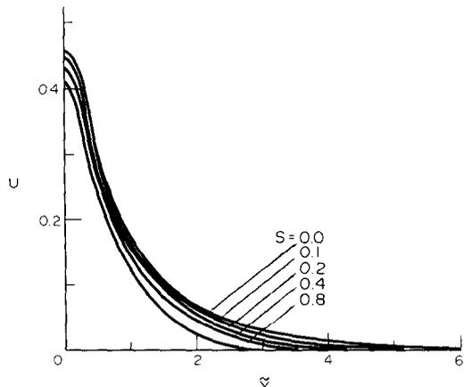
FIG. 8. Velocity distributions in the axisymmetric jet flow at  $Pr = 0.7$ ,  $X = 0.2$  and  $Gr/Re^2 = 0.47$  for various values of  $S$ .
