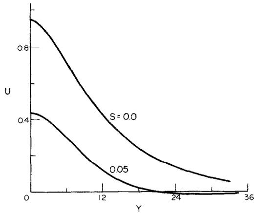
FIG. 4. Computed velocity profiles for the plume flow at  $Pr = 0.7$  and  $X = 100$ .
