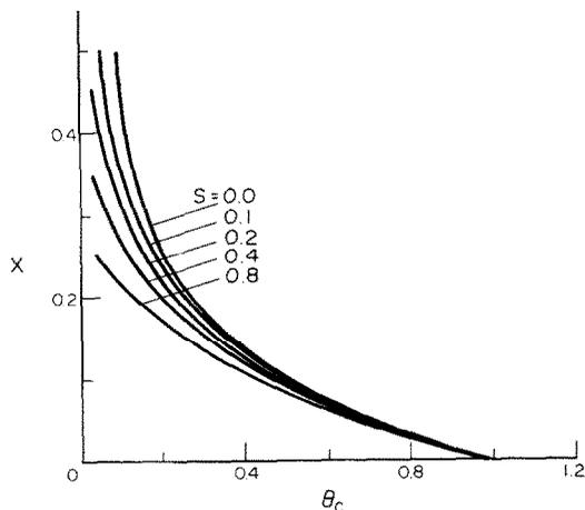
FIG. 10. Downstream centerline temperature variation in the buoyant jet flow at  $Pr = 0.7$  and  $Gr/Re^2 = 0.47$ .
